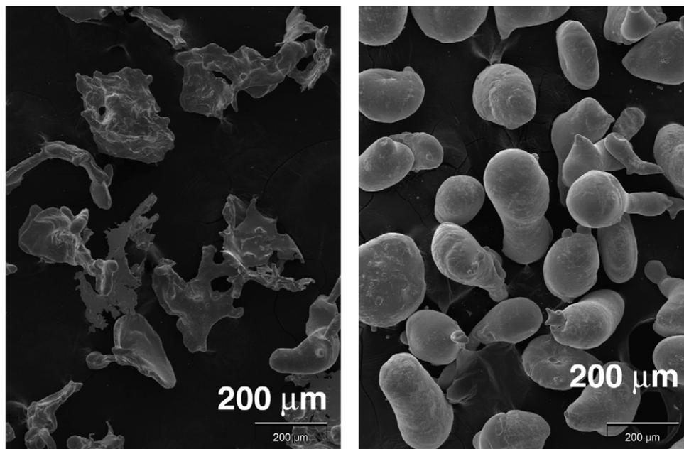
**Fig. 8 – Influence of the quenching liquid on the particle morphology: on the left, particles quenched into cold water and on the right, particles quenched into liquid nitrogen.**
