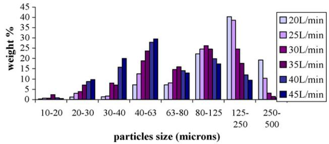
**Fig. 6 – Histogram for particle size distribution as a function of the atomising gas flow rate from 20 to 45 L/min (P = 3 bar).**
