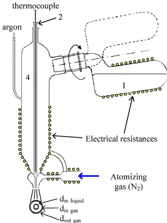
Fig. 1 – Experimental molten metal atomizer.
