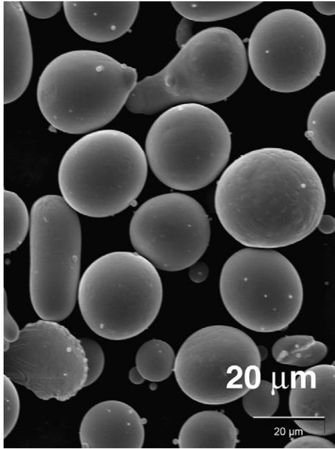
**Fig. 9 – Morphology of particles of 20–30  $\mu\text{m}$  (particles quenched into liquid nitrogen).**
