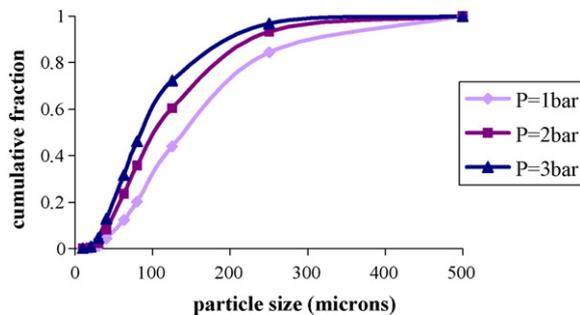
**Fig. 5 – Influence of the atomising gas pressure on particle size: cumulative fraction (experimental conditions: pressure of 1, 2 and 3 bar and gas flow rate of 30 L/min).**
