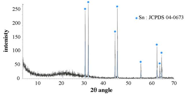
**Fig. 11 – X-ray diffraction diagram of atomised tin powder.**
