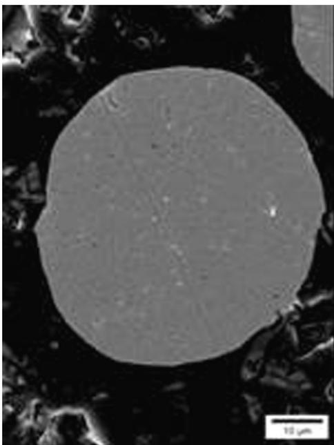
**Fig. 10 – SEM of a cross-section of a tin particle (40–63  $\mu\text{m}$ ).**
