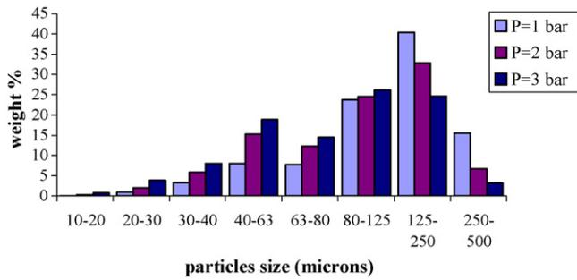
**Fig. 4 – Influence of the atomising gas pressure on particle size: histogram (experimental conditions: pressure of 1, 2 and 3 bar and gas flow rate of 30 L/min).**
