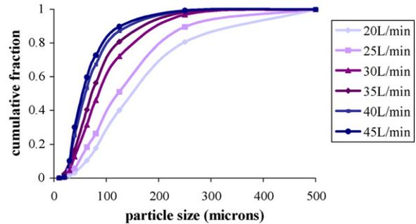
**Fig. 7 – Cumulative fraction for particle size distribution in function of the atomising gas flow rate from 20 to 45 L/min (P = 3 bar).**
