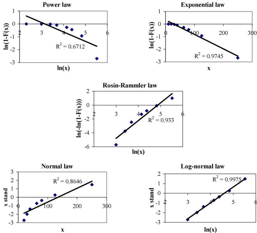
**Fig. 3 – Tests for approximation of particle size distribution to statistic laws (experimental conditions: pressure of 2 bar and gas flow rate of 30 L/min).**
