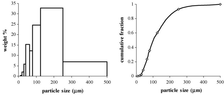
**Fig. 2 – Particle size distribution data: histogram and cumulative fraction representations (experimental conditions: pressure of 2 bar and gas flow rate of 30 L/min).**
