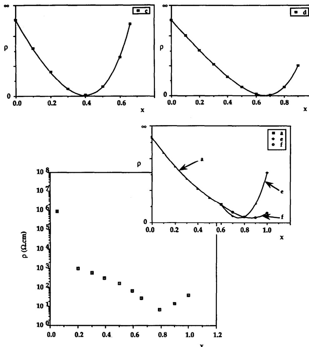
Fig. 2. □ Experimental change of resistivity as a function of the copper content  $x$ . Theoretical variation of the resistivity according to the cationic distributions: (a) with  $0 < x < 0.6$  plus (e) and (f) with  $0 < y < 0.4$ ; distributions (c) and (d) with Cu II in octahedral sites.
